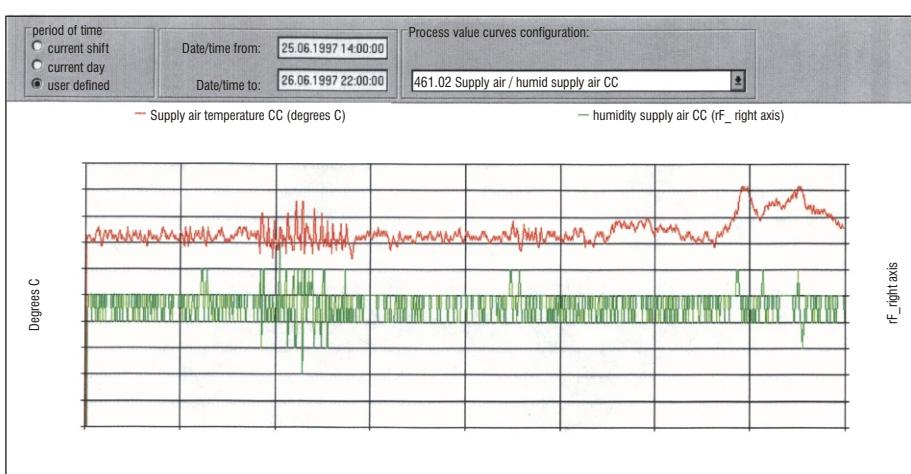
The diagram shows the low level of influence on the air condition parameters in the paint booth during cleaning operation process.
