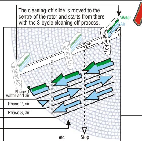
With THREE-PHASE TECHNOLOGY rotors can be excellently cleaned *during* operation of the ventilation plant.
