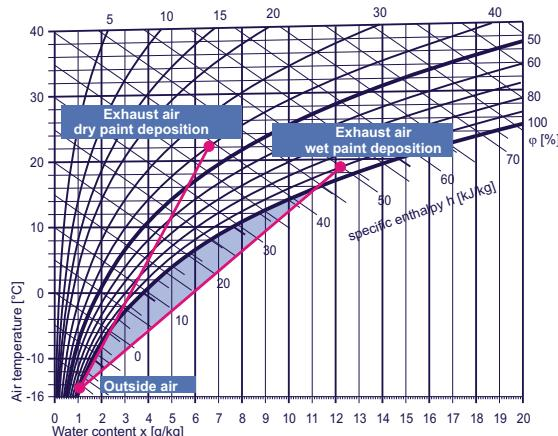
Higher exhaust air moisture produces more condensed water and excess water in the rotor.
