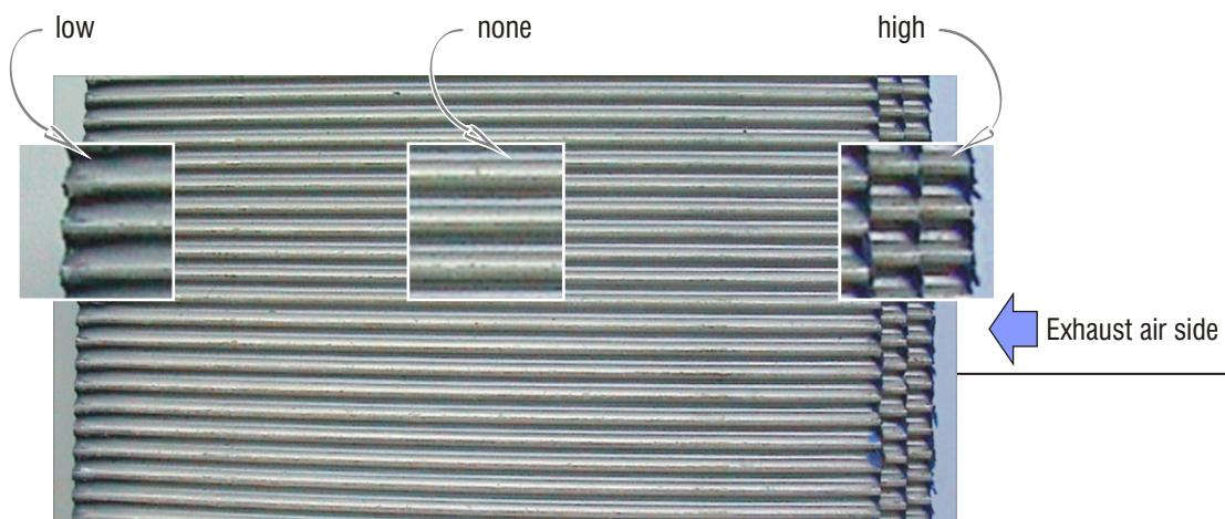
Due to the various paints and exhaust air treatment processes used in surface technology, the cleaning of the rotors demands the highest standards.
